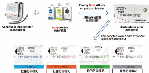
Nano ATE ink technology: double-layer-double-color printing effect 納米抗擦墨技術：雙層雙色打印效果
