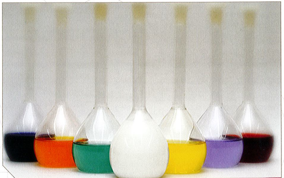
Regenerable nanosorbent (center) and its application in various types of dye-contaminated water.
